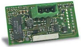
The Modbus RTU (RS485 communication) Card is a second Modbus RTU protocol available to select.
