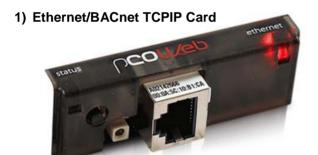
The Ethernet/BACnet TCPIP Card offer protocol option of:
