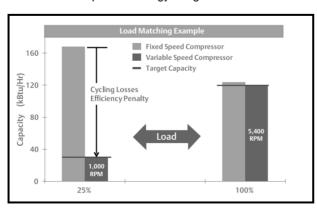
VFD Advantage 2 – Better temperature control compared to normal fix speed control.
