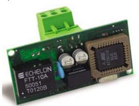
The LONWORKS Card is the protocol that was Created by Echelon Corp. The LONWORKS is a leading networking solution for building automation. The communication is based on the FTT10 electrical standard.
